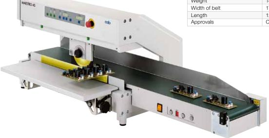
The correspondingly designated circular blade must be used for each different type of material that is to be cut.
