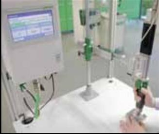
Adaptive screwdriving procedure DEPRAG CFC Clamp Force Control: Despite fluctuating tightening torques, the procedure guarantees reliable detection of the seating point and ensures a consistent final position for the subsequent final tightening resulting in a constant pre-load force.
